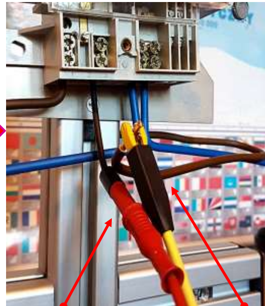
Connect safety plug and crocodile clip to phase and load current accordingly
