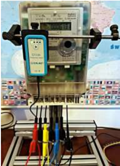
Connected meter ready for testing
