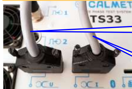
TS33 side clamps connection
