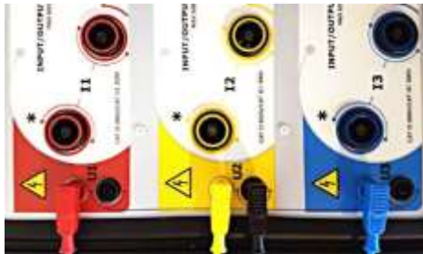
Voltage and clamps connection to the CT
