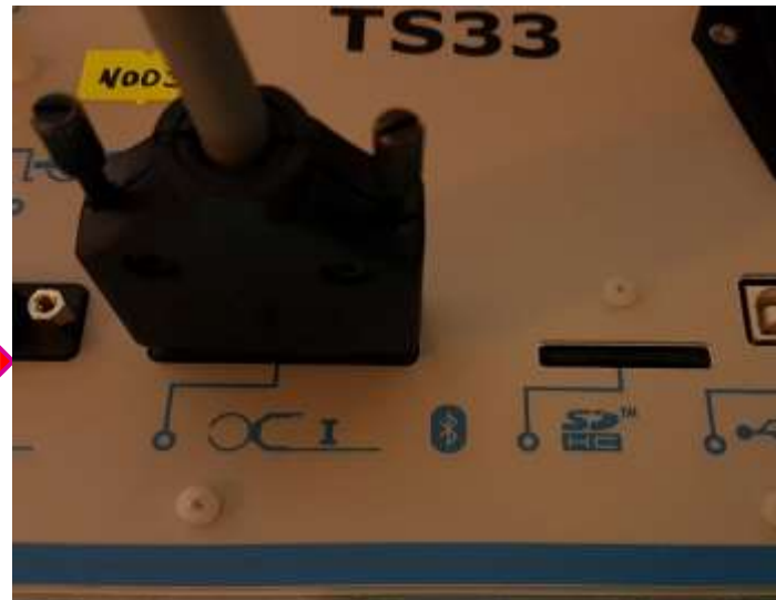
Connect current clamps plug into the socket on TS33. Clamp symbol appears on display.
