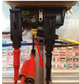
Connect return current cable by means of crocodile clip (black)
