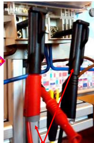
Connect voltage by safety magnetic plugs
