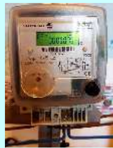
Typical single phase electronic meter with LED and its parameters
