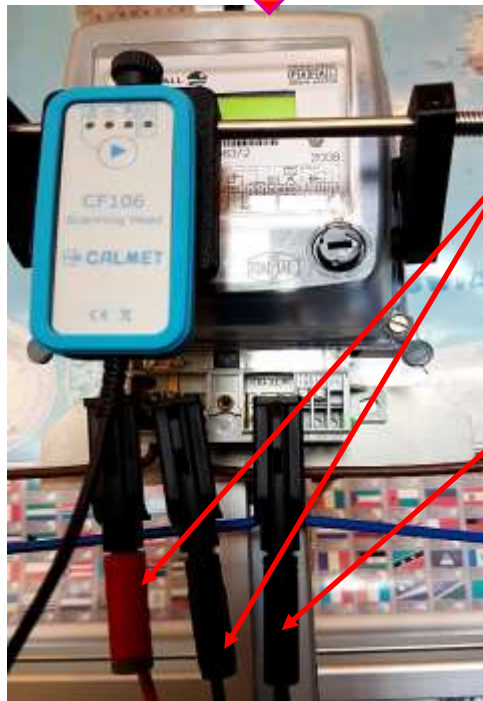
Typical single phase electronic meter with LED and its parameters
