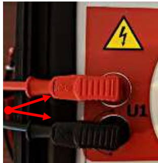
Connect cables from meter to voltage inputs of TS33
