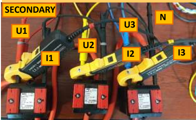
Voltage and clamps connection to the CT
