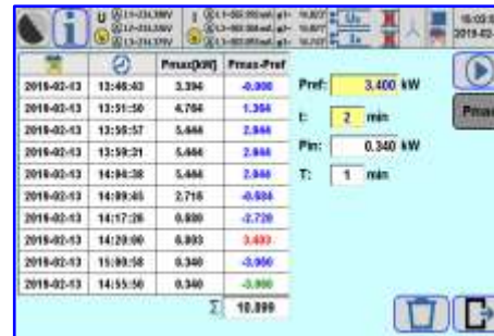
Maximum demand meter test
