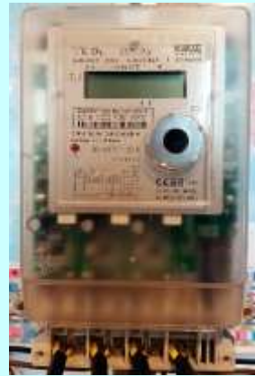
Typical three phase electronic meter with LED and its parameters
