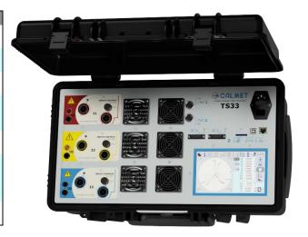
The Calmet TS33 portable test system consists of a three-phase reference meter of accuracy class 0.02% (or 0.04% or 0.1%) and an integrated three-phase current and voltage source up to 3x120A/600V. The TS33 is designed for analysis of complete metering installations and local mains conditions.
